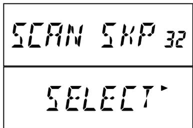
4. Press the [MHz(SETUP)] key, and then rotate the **DIAL** knob to select “SELECT”.
