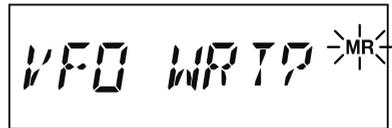
**Note:** If a split Frequency Memory channel was transferred, the TX frequency will be ignored (The transceiver will be set up for Simplex operation on the Receive frequency.)
