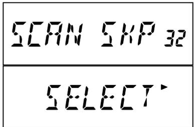
4. Press the [MHz(SETUP)] key, and then rotate the **DIAL** knob to select “SELECT”.
