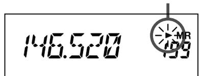
A blinking “▶” icon will appear when you recall the “skipped” memory channel manually. To reinstate a channel into the scanning loop, select “OFF” in step 4 above, after first recalling the currently blocked channel (the “Skipped” channel is accessible via manual channel selection methods using the **DIAL** knob in the Memory mode, whether or not it is locked out of the scanning loop).
